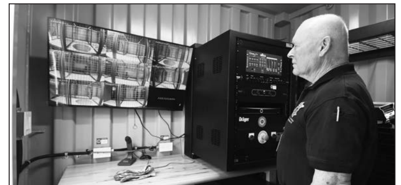
Advanced Fire Skills Program Coordinator Al Beardsley stands in the new SCBA Maze Trailer’s control room, which features a digital audio and video feed from multiple cameras inside the training area. Instructors can communicate with trainees and control lights and sound at all times.
